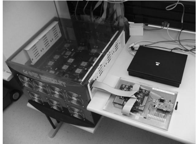
Figure 2: Complete BPU with a radio front-end
